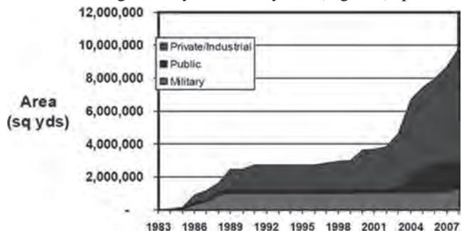
Fig. 3.1—Increasing use of RCC pavements (Pitman and Anderton 2009). (Note: 1 yd<sup>2</sup> = 0.8 m<sup>2</sup>.)
