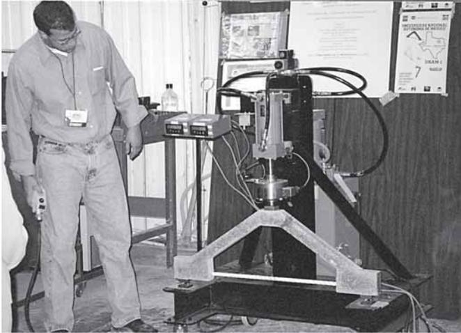
Student competitions, a regular event at conventions, have featured the building and testing of a wide variety of concrete projects: cubes, beams, bowling balls, and egg-protection devices. Pictured is the testing of a fiber-reinforced polymer concrete frame in a 2001 competition.
