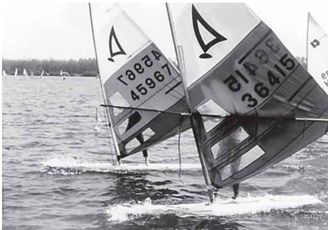
The first concrete windsurfer race was held at Den Bosch, The Netherlands, in 1985. One board was built from ferrocement and one from glass-reinforced concrete (GRC).
