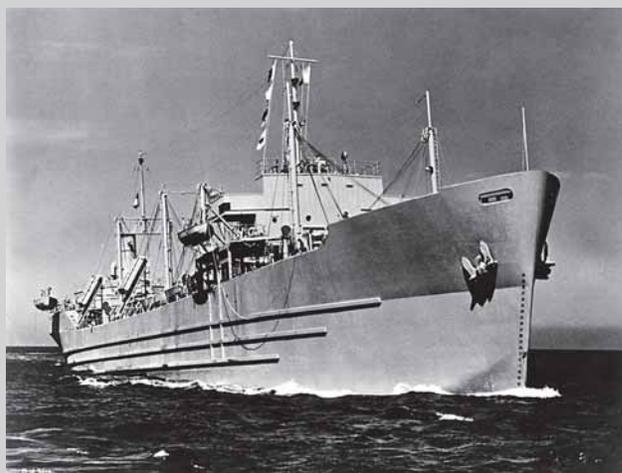
Dry-cargo, self-propelled concrete ship built during World War II by U.S. Maritime Commission. The hull shell was 6-1/2 in. (165 mm) and contained from three to five layers of closely-spaced reinforcing. Cover over the steel was 3/4 in. (19 mm) on the outboard face and 1/2 in. (12 mm) on the inboard face.
