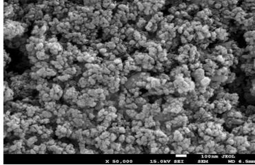
Fig 6.1 Nano  $\text{Al}_2\text{O}_3$
