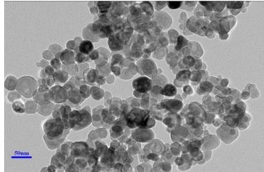
Fig 6.2 Nano  $\text{Fe}_2\text{O}_3$
