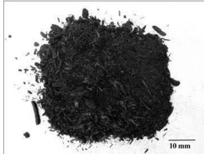
Fig 4.1 Sugarcane bagasse ash
