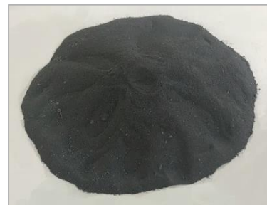
Figure 1: Grey densified silica fume
