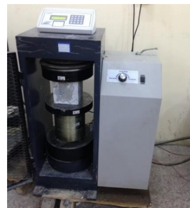
Figure 9: Compressive strength machine
