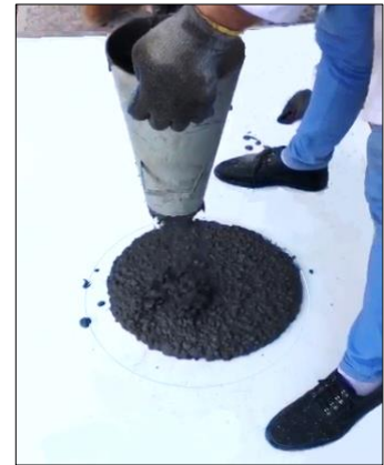
Figure 4: Slump flow test
