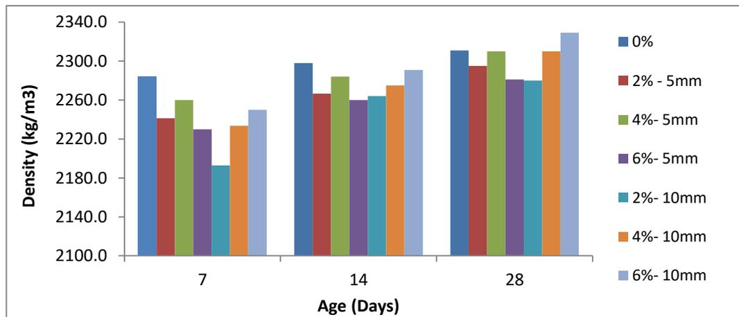
Fig. (6) The effect of rock wool on density of ferrocement mortar with water curing.
