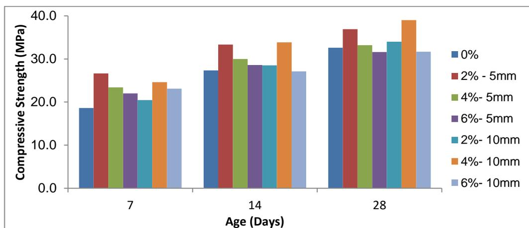
Fig. (8) The effect of rock wool on compressive strength of ferrocement mortar with water curing.
