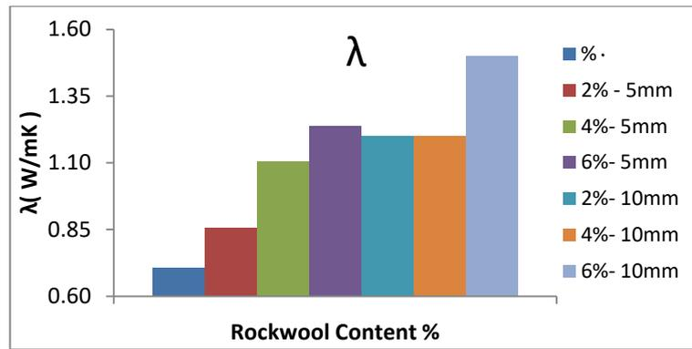
Fig. (14) The effect of rock wool on thermal conductivity of ferrocement mortar using CO<sub>2</sub> curing.
