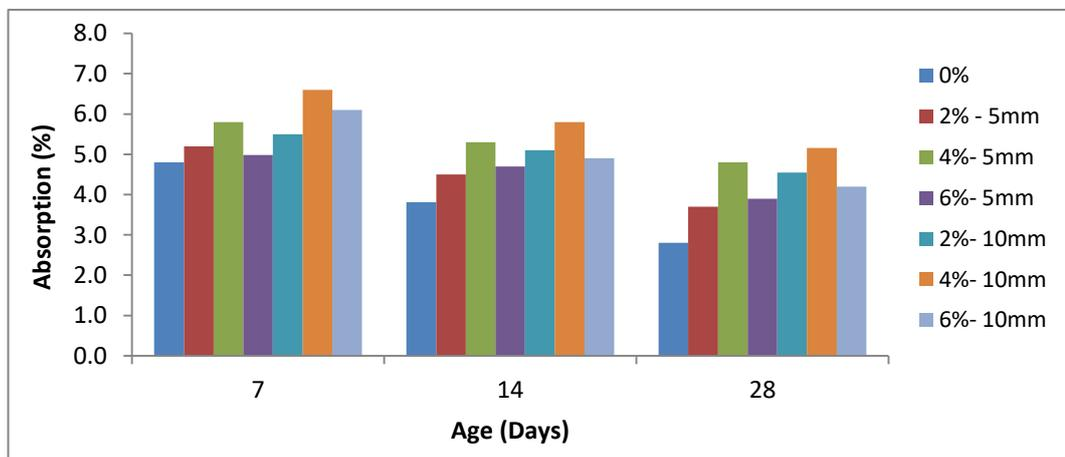
Fig. (17)The effect of rock wool on absorption of ferrocement mortar using CO<sub>2</sub> curing.
