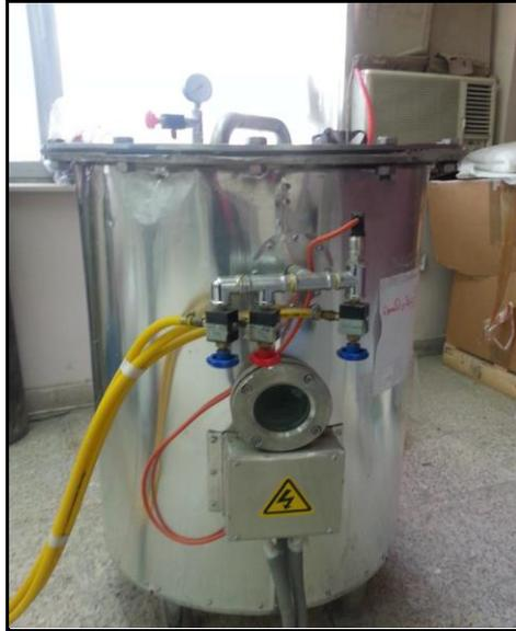
Fig. (2) Carbonation chamber machine
