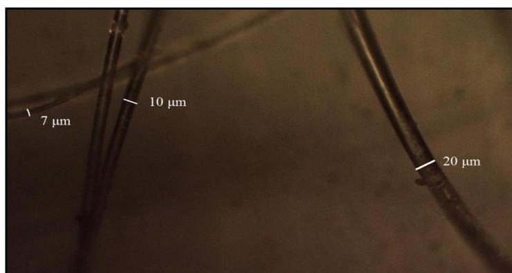
Figure (1) Diameter of rock wool
