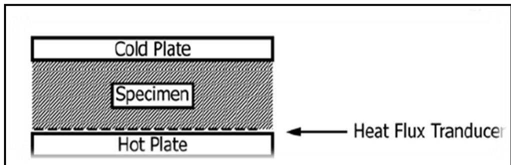
Fig. (5) Apparatus with One Heat Flux Transducer and One Specimen
