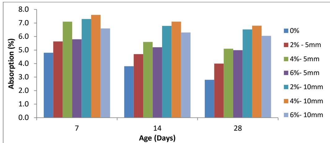
Fig. (16)The effect of rock wool on absorption of ferrocement mortar using water curing.
