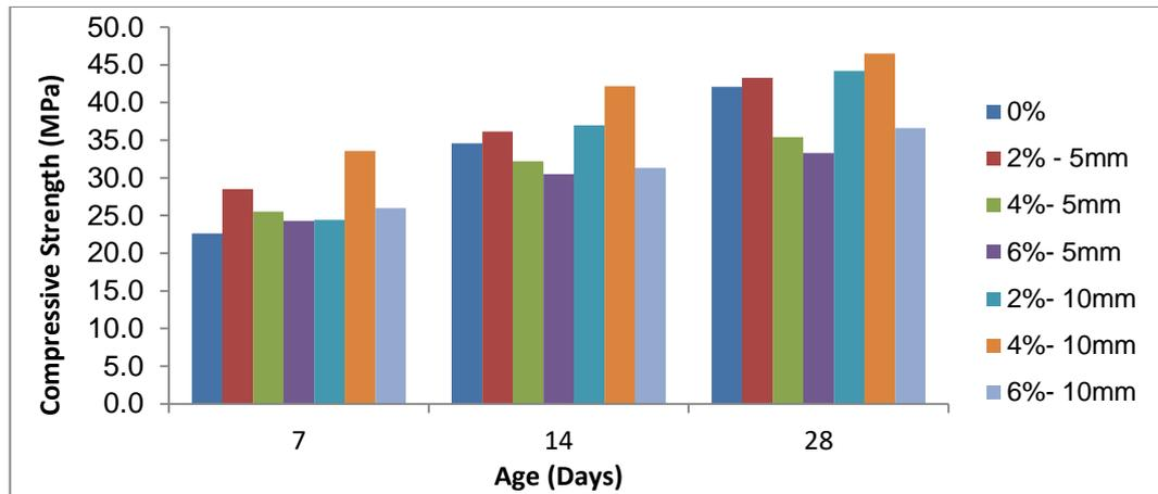
Fig. (9) The effect of rock wool on compressive strength of ferrocement mortar with CO<sub>2</sub> curing.
