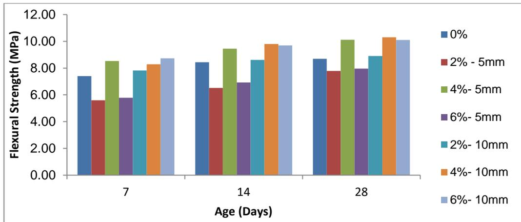
Fig. (10) The effect of rock wool on flexural strength of ferrocement mortar using water curing.
