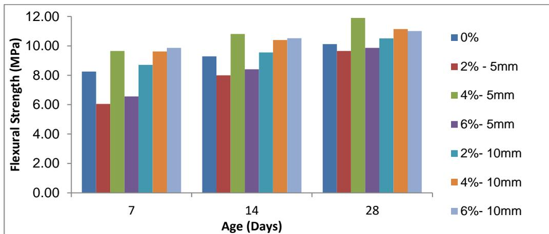
Fig. (11) The effect of rock wool on flexural strength of ferrocement mortar using CO<sub>2</sub> curing.
