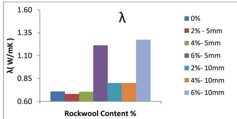
Fig. (12) The effect of rock wool on thermal conductivity of ferrocement mortar using water curing.
