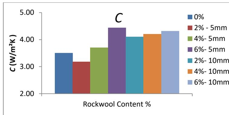
Fig. (13) The effect of rock wool on thermal conductance of ferrocement mortar using water curing.
