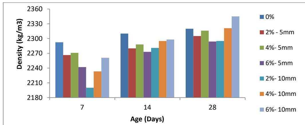
Fig. (7) The effect of rock wool on density of ferrocement mortar with CO<sub>2</sub> curing.
