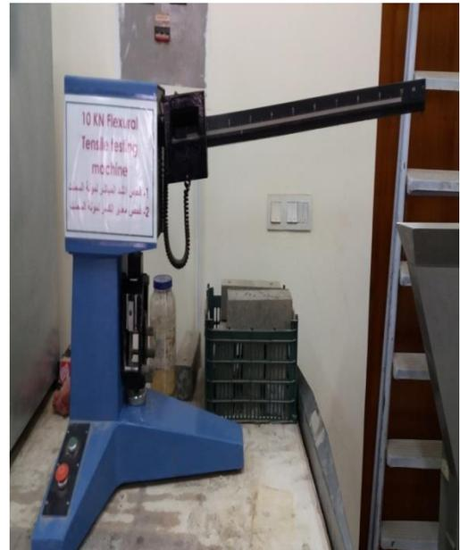
Fig.(3) Compressive Strength Test      Fig.(4) Flexural Strength Test
