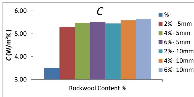
Fig. (15) The effect of rock wool on thermal conductance of ferrocement mortar using CO<sub>2</sub> curing.
