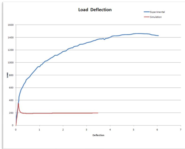
**Figure 5**– Fitting of  $\epsilon_{cr}$  to load deflection curve
