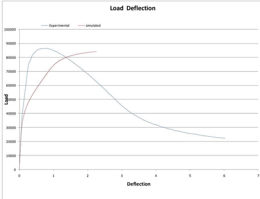
**Figure 16** – Linear section of load deflection clearly modeled by  $E=20000$  MPa.
