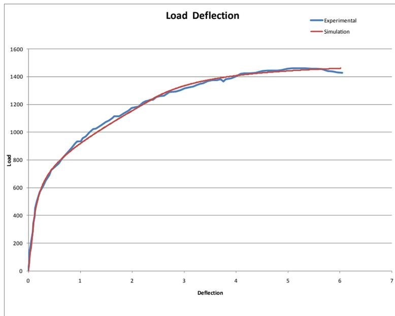
**Figure 9** – Load deflection curve response to change in  $\beta_{tu}$ .
