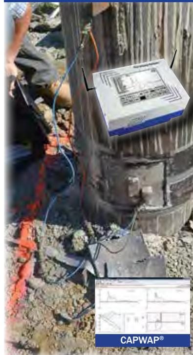
The best system for Dynamic Load Testing of any type of deep foundation.
