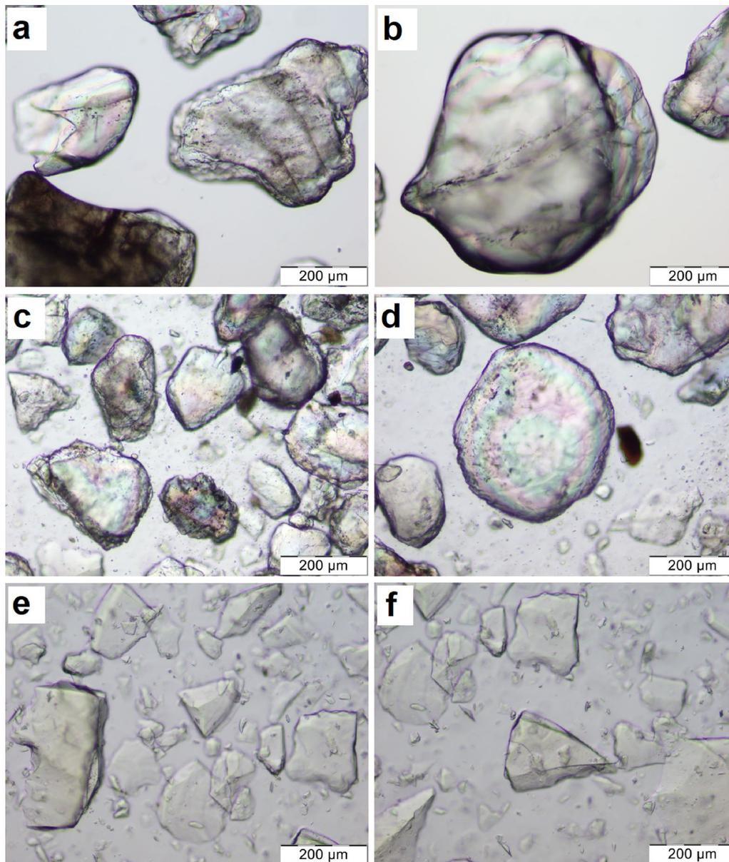
**Fig. 2** Optical images of quartz sand (a–b), dune (desert) sand (c–d) and crushed glass (e–f)
