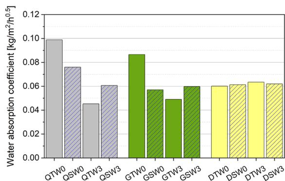
**Fig. 10** Water absorption coefficient of different LWAC mixes
