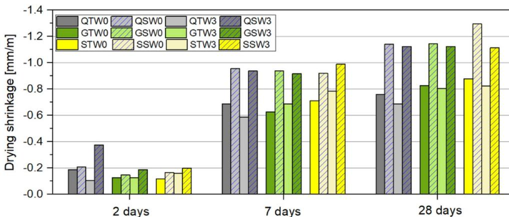
**Fig. 12** Measured drying shrinkage of LWAC at different ages
