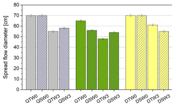
**Fig. 6** Slump flow results of different concrete mixes according to EN 12350-5
