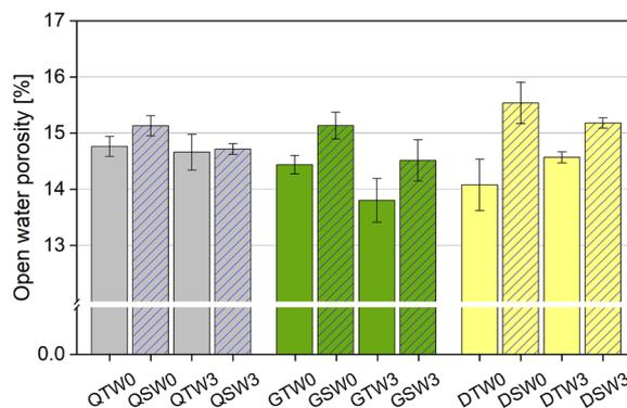
Fig. 9 Capillary water porosity of LWAC mixes
