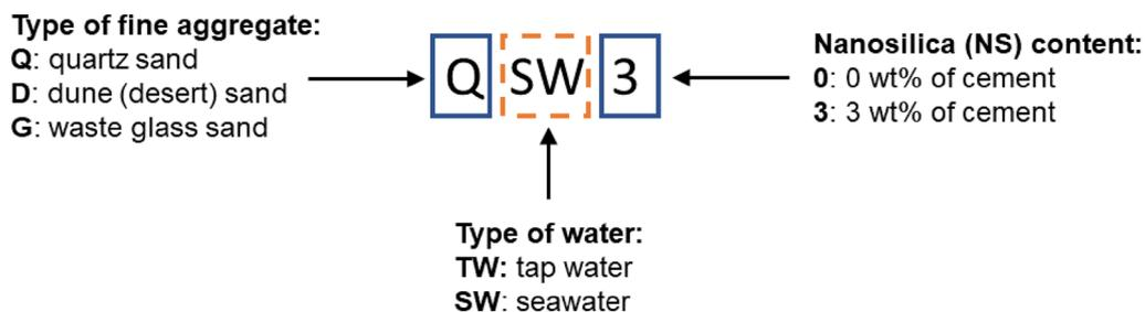
**Fig. 3** Graphical description of specimens' designation
