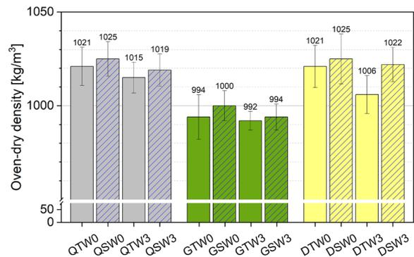
**Fig. 7** Measured oven-dry density of different LWAC mixes
