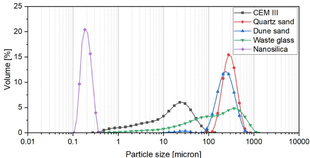
**Fig. 1** Particle size distribution of the used fine materials
