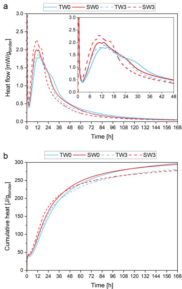
**Fig. 5** Hydration heat (a) and cumulative heat (b) of cement pastes produced with and without seawater and nanosilica
