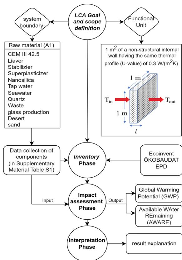
Fig. 4 The schematic figure for LCA in this study
