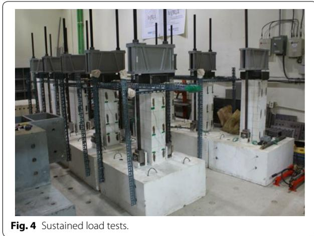
concrete placement (i.e.  $t_0=37$  days). The tests were carried out during winter season in Korea. As shown in Fig. 4, the column specimens were placed in the basement laboratory where the variation of temperature and relative humidity between day and night was relatively insignificant. The average temperature and relative humidity of the basement laboratory during the sustained load tests were approximately 8 degrees Celsius and 40%, respectively.
