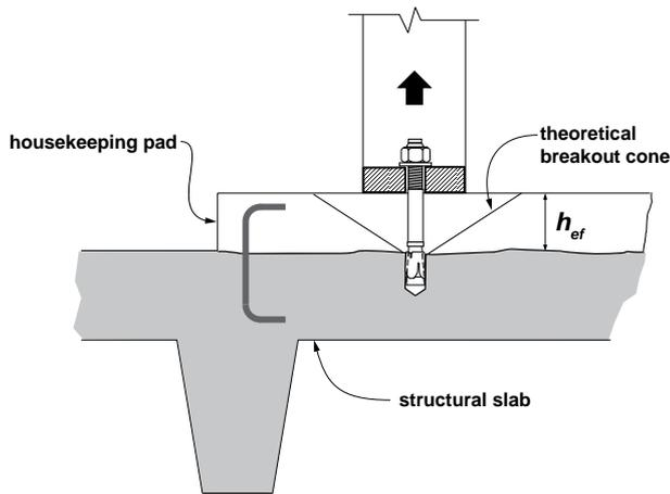
Fig. 1: Expansion anchor in a housekeeping pad with marginal penetration into the structural slab below ( $h_{ef}$  is the effective embedment depth that should be assumed for this case)
