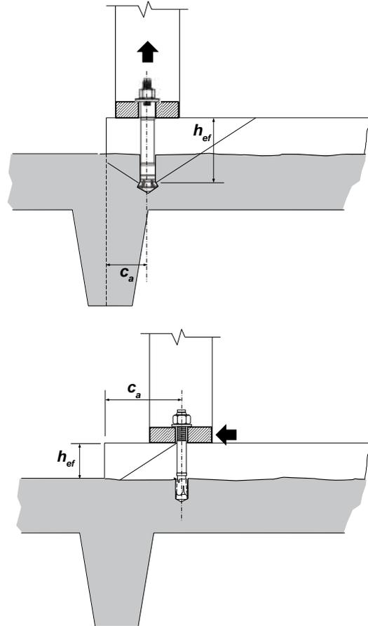
Fig. 3: A full-depth breakout cone may not develop for near-edge anchors. Tension or shear breakout capacities may be limited by the distance  $c_a$  measured from the centerline of the anchor to the edge of the housekeeping pad
