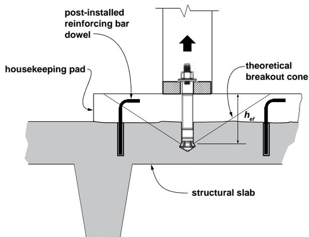
Fig. 2: Undercut anchor in a housekeeping pad anchor with substantial engagement (at least three anchor diameters) into the slab below. Here, post-installed dowels are used to anchor the pad to the structural slab
