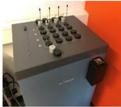
Isoth. Calorimetry at 40°C
