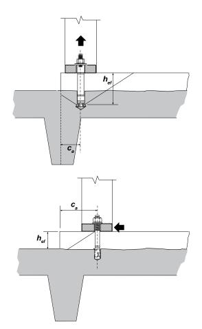
Fig. 3: A full-depth breakout cone may not develop for nearedge anchors. Tension or shear breakout capacities may be limited by the distance  $c_a$  measured from the centerline of the anchor to the edge of the housekeeping pad
