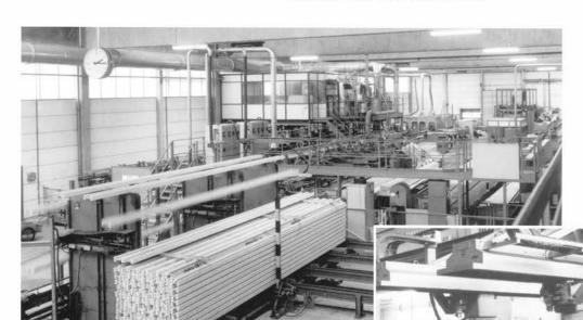
**1-2** Automated construction lines are common for formwork production, just as for other industrial assembly work. Welding robots are shown fabricating metal frames used for heavy panels. The upper picture shows fabrication of wood I-beam form supports. In an alternative approach to efficient fabrication, components of job-built forms are precut and shipped to the job site for assembly (see Figure 3-2).
