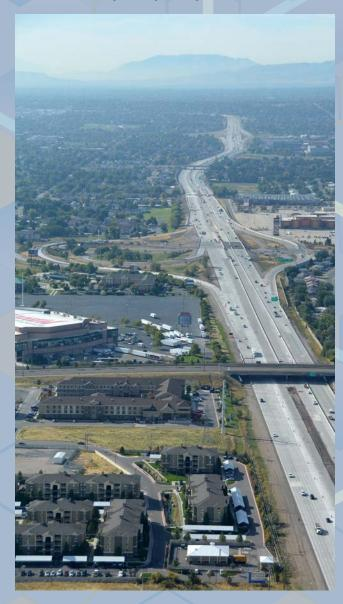
The reconstruction of 7 miles (11 km) of I-215, encompassing over 43 lane miles (69 km), replaced aging pavement with high-quality, durable concrete. The project's seven bridges each received various treatments, such as new superstructure, widening, and hydro-demolition. Concrete used on the decks was reinforced with both macro and micro fibers. The bridge at SR-201 used a lightweight fiber-reinforced concrete deck.
