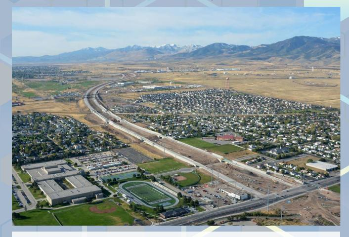
This project added 2 miles (3 km) of outside freeway lanes, 14 mainline bridges, seven pedestrian bridges, walls, a single-point urban interchange, and a shared-use path, encompassing over 40,000 yd³ (30,580 m³) of concrete. Steel fiber reinforcement was used on two bridges, the first application of this technology on a bridge in the United States.
