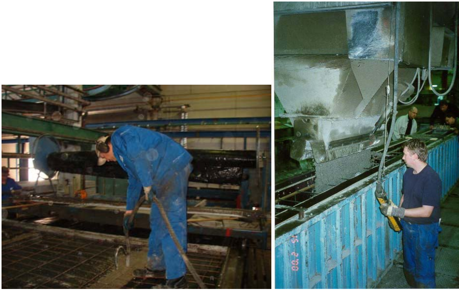
Fig 14 - From noise, vibration, ergonomic loading to high quality working environment using SCC in precasting (Courtesy of K. Juvas)
