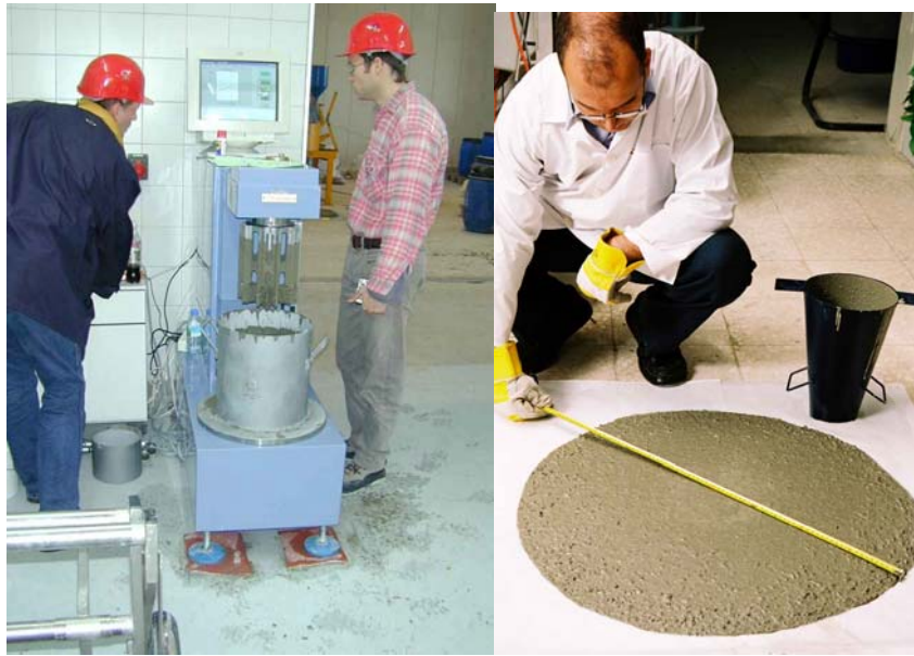
Fig 3 - Viscometer used for determining rheological material data and workability testing in practice (Courtesy of M. Sonebi).
