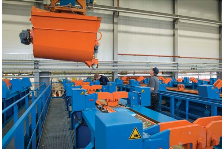
Fig 13 - Walls being cast with SCC as an integrated part of the fully industrialised prefabricating house building system NCC complete (Courtesy of NCC, Sweden)
