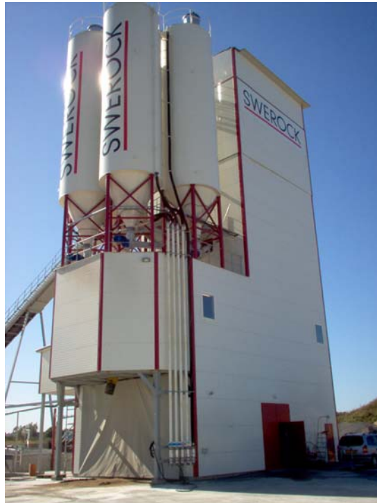
Fig 4 - A modern concrete mixing plant with several silos (Courtesy of Swerock, Sweden).
