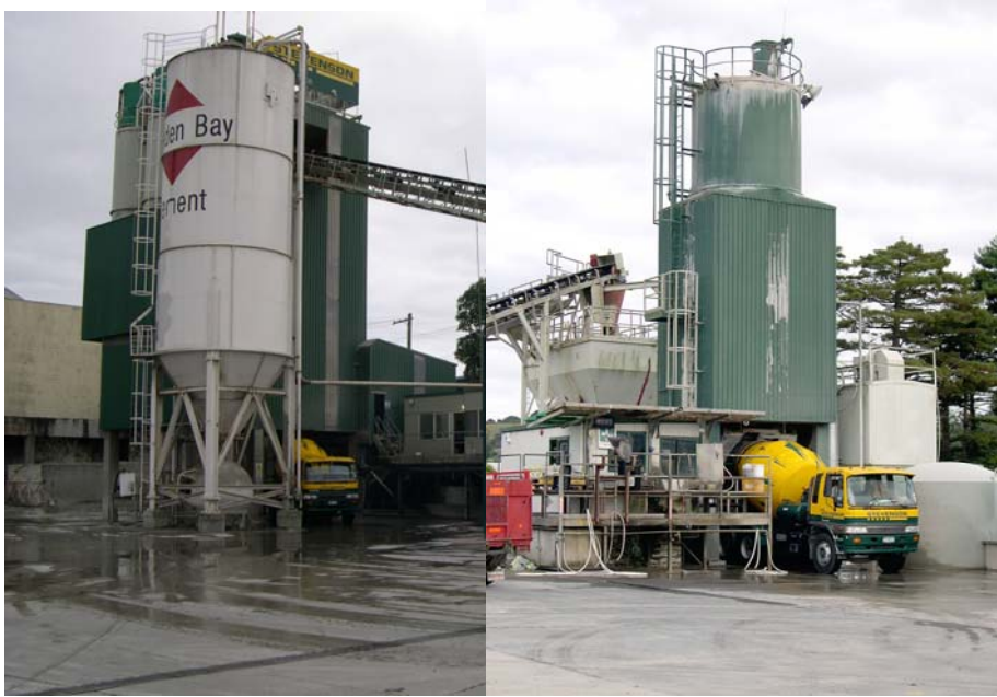
Fig 6 - Both factory mixing and truck mixing is viable for SCC (Courtesy of M. Khrapko)
