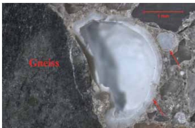
Fig. 5: Alkali-silica gel (red arrows) in voids near reactive gneiss particle
