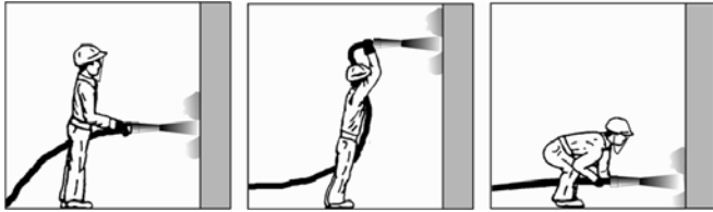
Fig. 8.3(a)—Correct gunning positions. Correct shooting position is to hold nozzle at 90 degrees (perpendicular) to surface.
