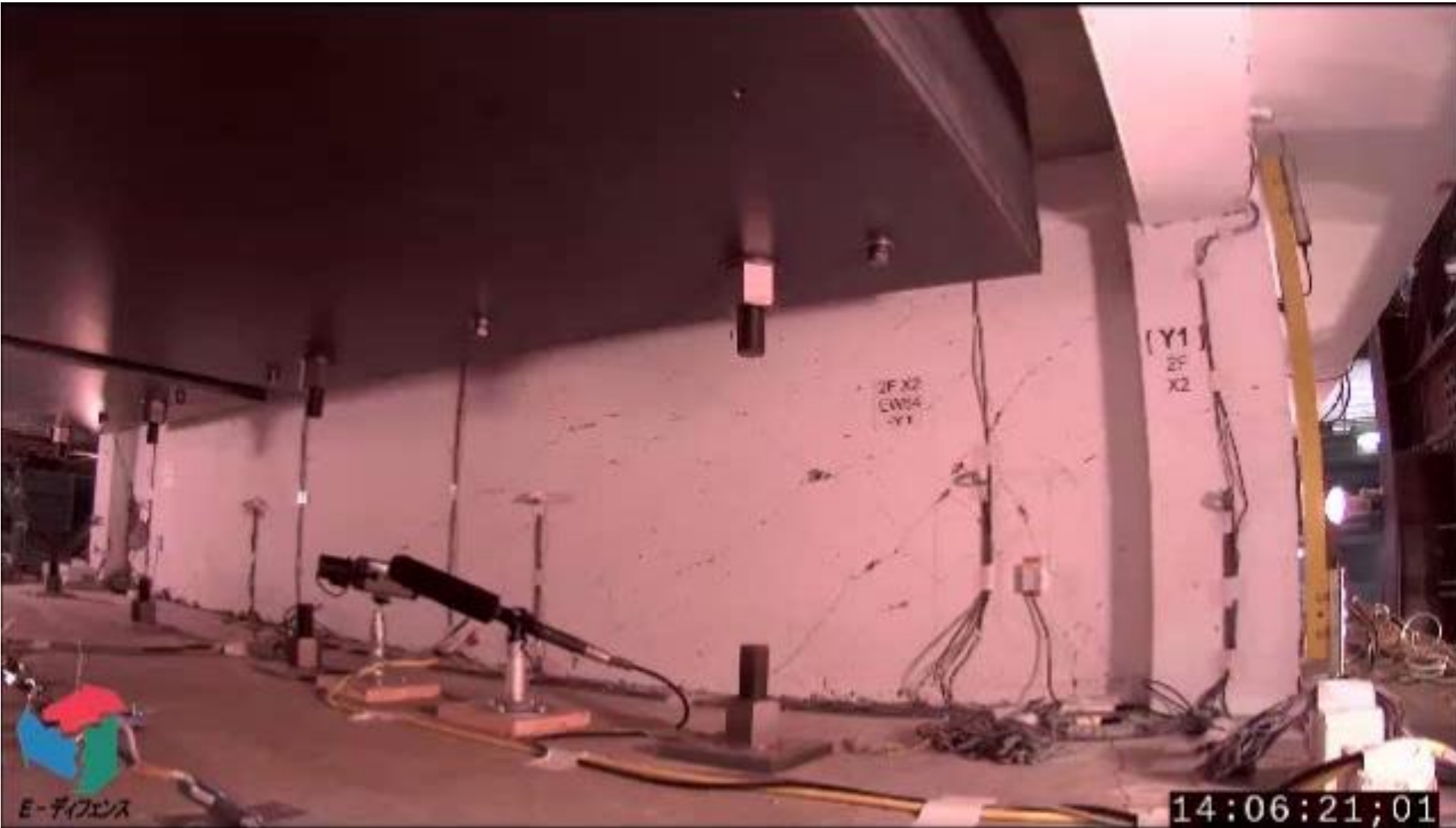
#3-5(JMA Kobe 140%-1) 1/2 wall in X-2 frame on the 2nd floor
