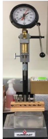
Setting time test by penetration resistance
