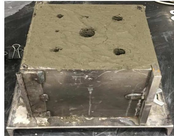
Setting time test by penetration resistance
