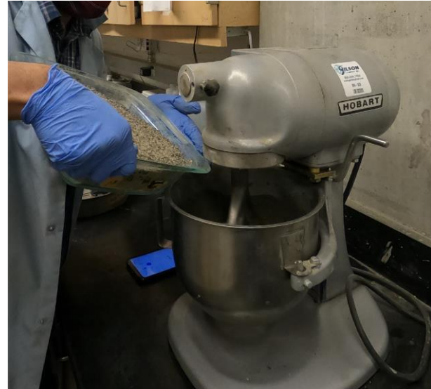
Preparation of mortar using a benchtop mixer
