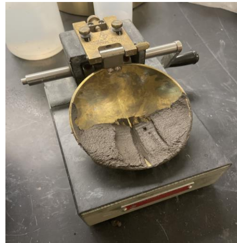
Casagrande (left) and plastic roller (right) used in Atterberg tests
