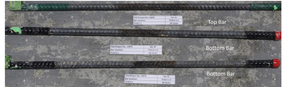
Typical CAC2 showing corrosion on top and bottom bars
