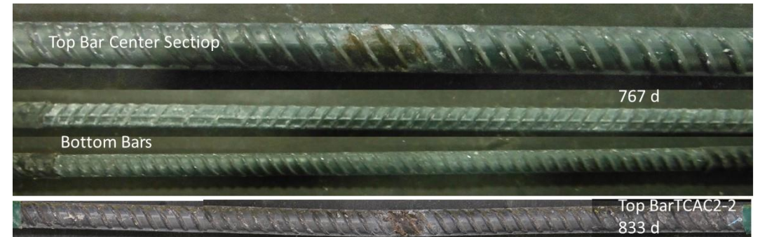
Typical CACT showing corrosion on top but not bottom bars
