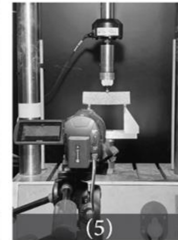
Three-point bending schematic test setup (1), the cross-section of the tested beam (2), primary 3D Printed slab of 100×350×50 mm with 20 mm circular nozzle (3), four extracted 140×40×40 mm beams from the primary slab (4), the third point bending test setup (5)
