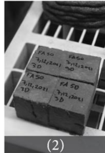
Primary 3D printed 150×150×60 mm sample with 20mm circular nozzle (1), four extracted 50×50×50mm cubic specimens from the primary sample (2), Compressive test setup with samples tested perpendicular to the loading direction (3)
