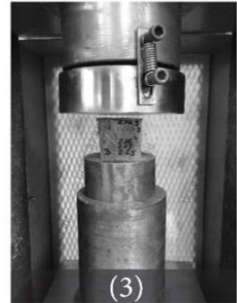
Primary 3D printed 150×150×60 mm sample with 20mm circular nozzle (1), four extracted 50×50×50mm cubic specimens from the primary sample (2), Compressive test setup with samples tested perpendicular to the loading direction (3)
