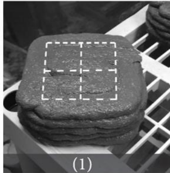
Primary 3D printed 150×150×60 mm sample with 20mm circular nozzle (1), four extracted 50×50×50mm cubic specimens from the primary sample (2), Compressive test setup with samples tested perpendicular to the loading direction (3)
