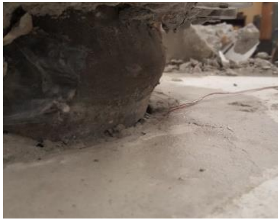
12.45% Drift Ratio (significant buckling of the steel pipe)
