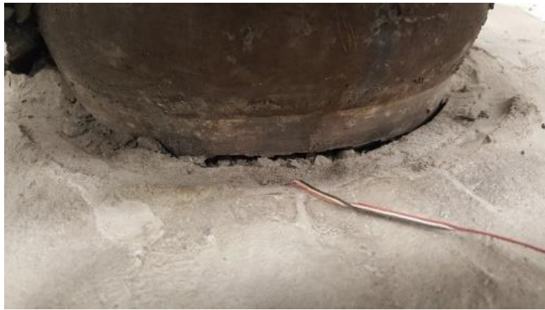
12.45% Drift Ratio (significant buckling of the steel pipe)
