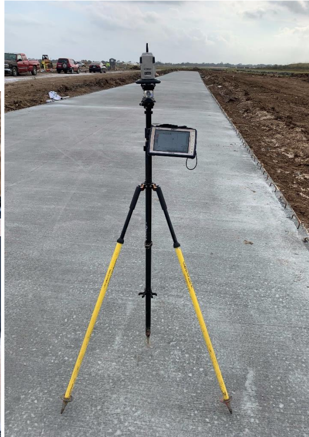
Prism and rod actively measuring a location from the data collector
