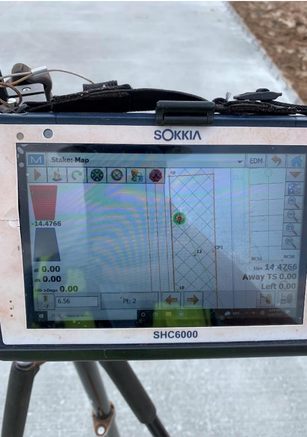
Prism and rod actively measuring a location from the data collector
