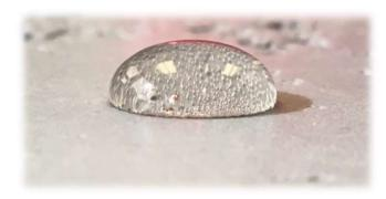
Concrete with Colloidal Silica
