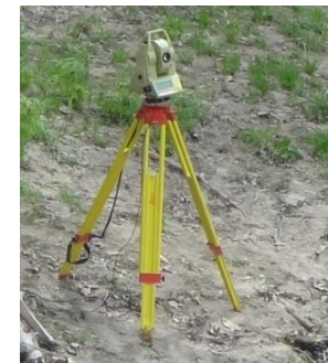
Automated Total Station
