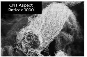
Bundle L ≥ 10 µm D: 1-2 µm Tubes D: 10+/- 2 nm
