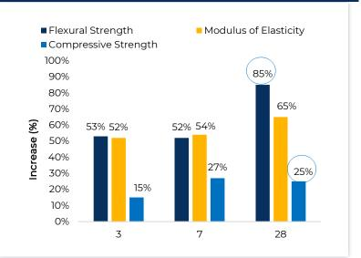
0.20 % MWCNT on Cement Portland I/II, 72 % MWCNT in NTeC-C MWCNT Bundle
