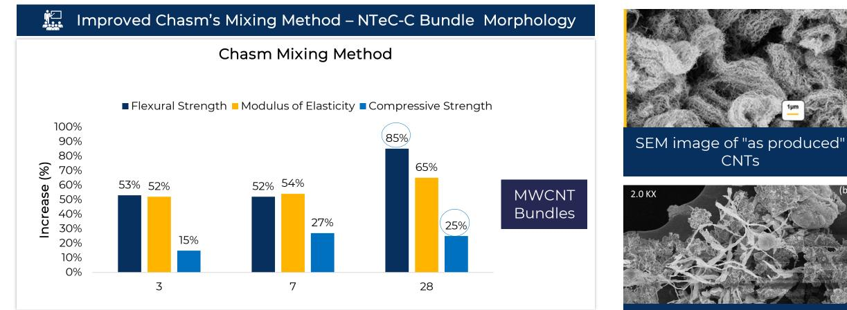
0.20 % MWCNT on Cement Portland I/II, 72 % MWCNT in NTeC-C MWCNT Bundle Morphology
