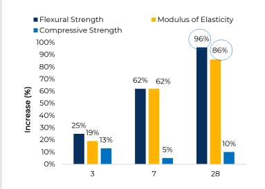
0.10 % MWCNT on Cement OPC-I, 68 % MWCNT in NTeC-C MWCNT Bundle
