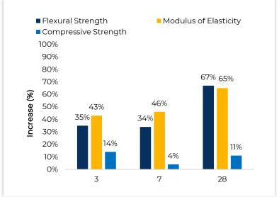
0.10 % MWCNT on Cement OPC-I, 60 % MWCNT in NTeC-C MWCNT Bundle
