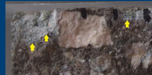
White silver nitrate precipitate forms on the part of the face where chloride ions are present
