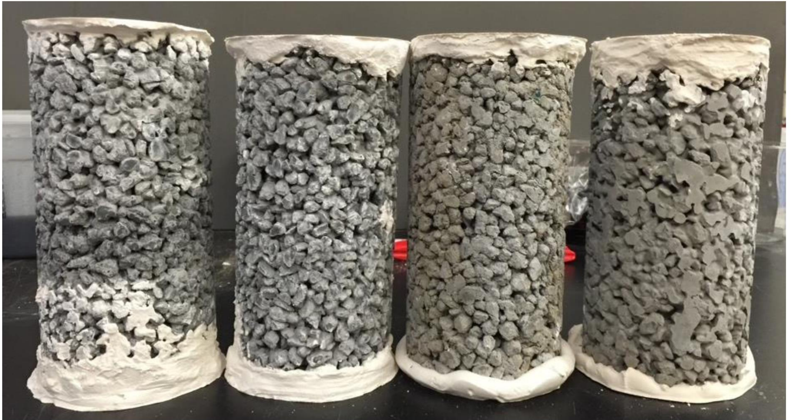
Figure 4.1 Pervious concrete cylinders with capping: (left to right) cement, cement + GO, fly ash, fly ash + GO
