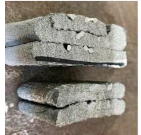
Weak bonds and cold joints
