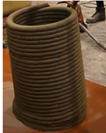
Plastic collapse Concre3DLab Ghent
