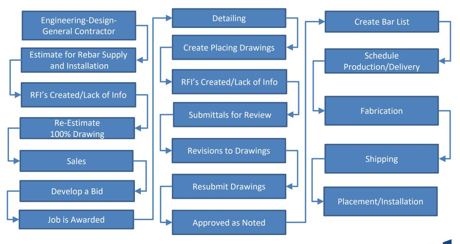
Need to go from a fragmented, linear process (engineering to construction) to...
