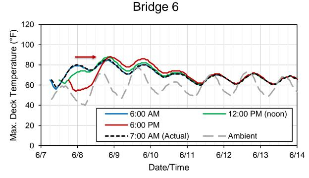
Placing concrete in late afternoon shifts peak temp. difference to Day 2 or 3.
