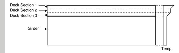
Creep was implicitly modeled by reducing the elastic modulus of concrete
