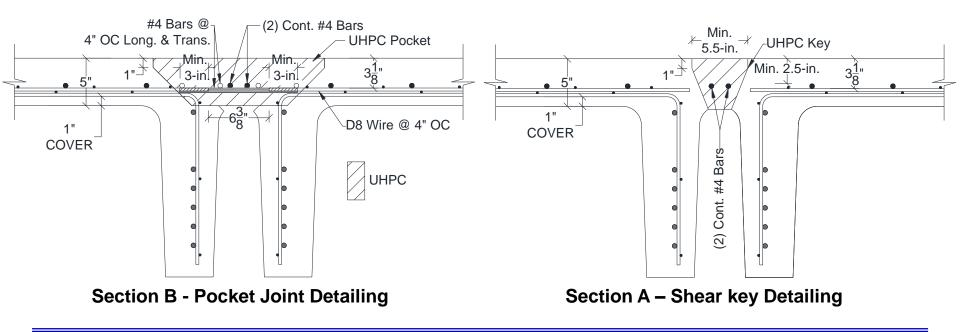
Rehabilitation of Longitudinal Joints in Double-Tee Bridge Girders
