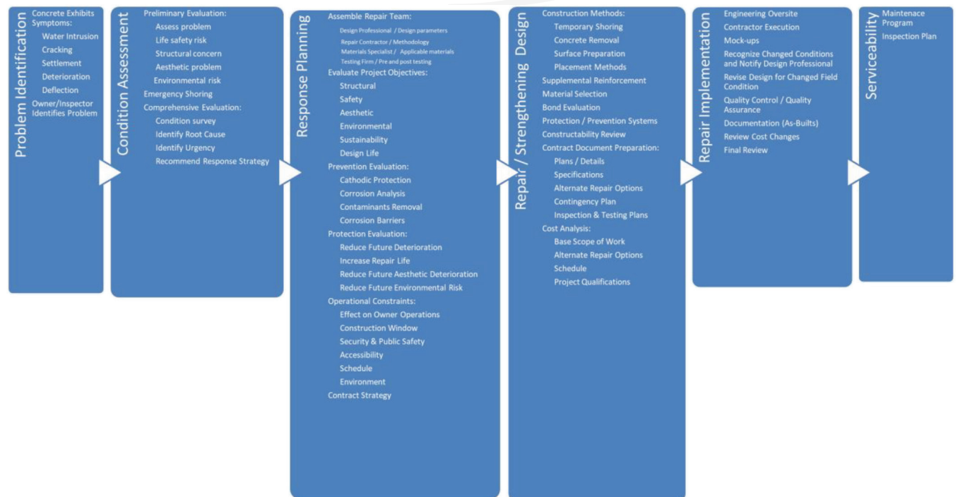
Fig. 3.1—Concrete repair/strengthening process.
