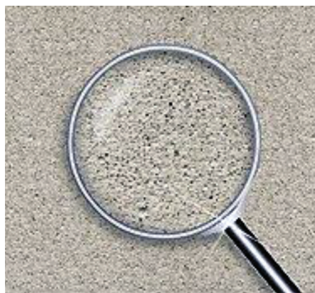
Fig. 1.3—Macroscopic cellular (void) structure of AAC.
