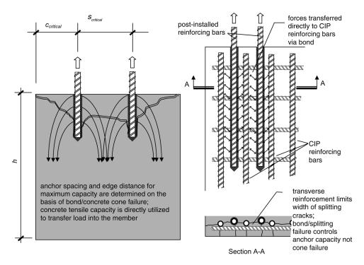
(a) Reinforcing dowels designed using anchor theory as addressed by this criteria.
