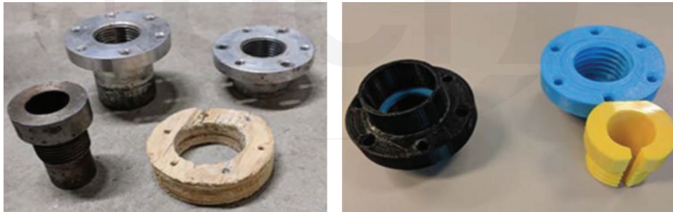
Fig. 7.1b—Pressure sensor adaptors.
