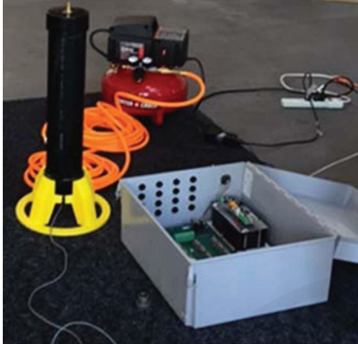
Fig. 7.1a—Calibrating pressure sensors and data acquisition system.
