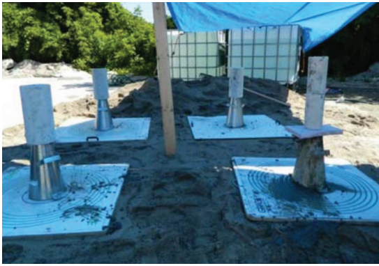
Fig. 8.1b—Concrete characterization using slump flow loss test.
