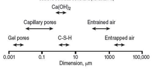
Fig. 3.3.1a—Relative sizes of different types of pores and other microstructural features (adapted from Mehta [1986]).
