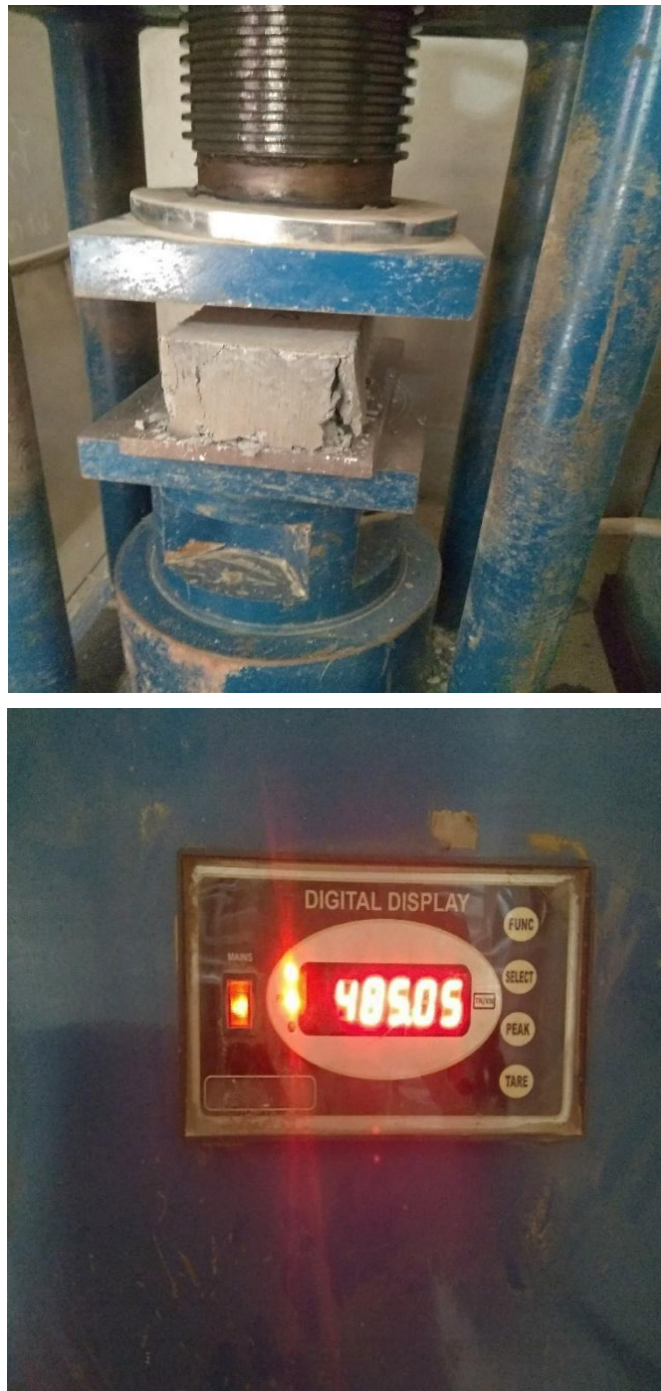
Figure 4. 1: Compressive strength test
