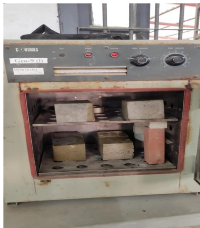
Figure 4.6: Concrete specimen kept in oven for water absorption test
