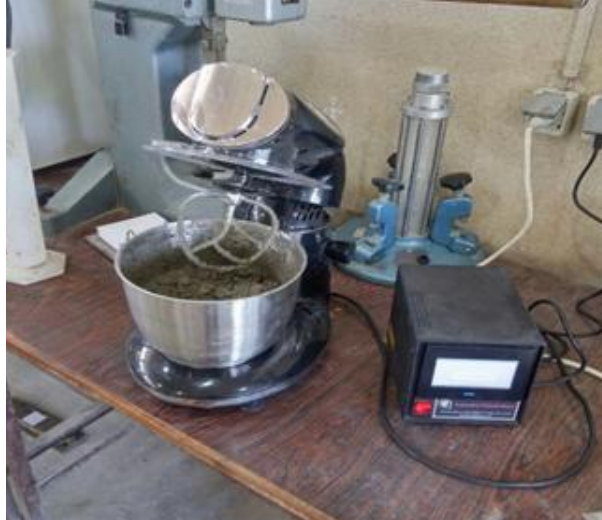
Fig. 2. A view of mortar mixer machine
