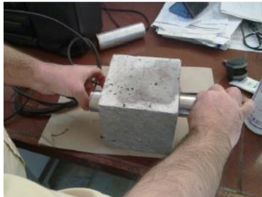
Fig. 2. Direct method to measure the pulse velocity in concrete samples
