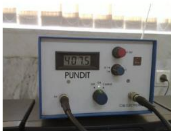
Fig. 1. PUNDIT device to measure the ultrasonic pulse velocity in concrete samples
