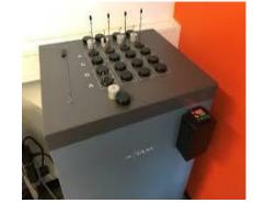
Isoth. Calorimetry at 40°C
