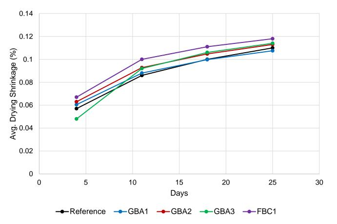
Tested according to ASTM C596 • w/cm kept at 0.44 - to match the value used in concretes
