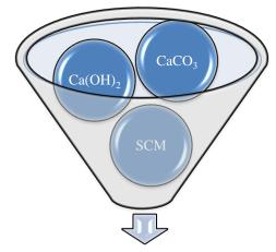
Mixed for 4 mins and sealed cured at 40°C
