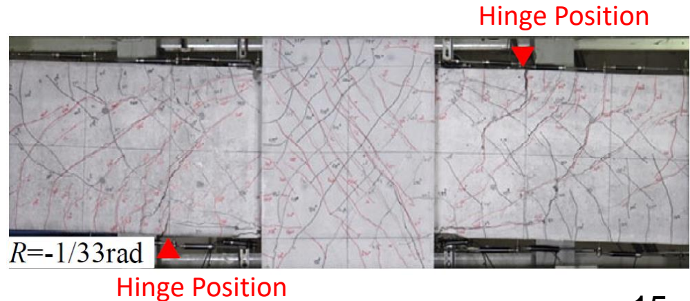
Crack Condition after Large Deformation
