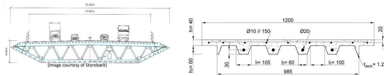
Suspension bridge decks are designed to be light in weight to reduce deadload on the suspension cables and stiff to resist movement (bending & torsion) from wind and traffic. This results in very thin composite decks, with a potential for punch through if too much of the existing concrete material is removed during rehabilitation.
