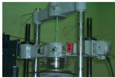
Bar Rupture with 4 d<sub>b</sub> in UHPC @ 14,000 psi.
