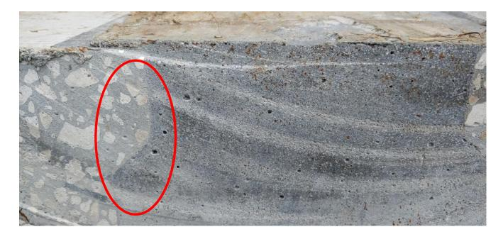
**UHPC Interface Bond to Normal Concrete.**
