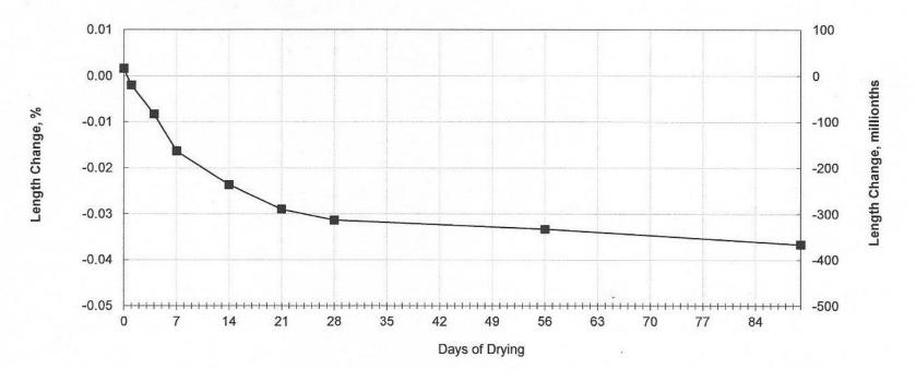
ASTM C1107/C1107M-20 specifies that a Nonshrink Hydraulic Cement Grout shall not have a change in length of more than 0.3% at 28 days.
