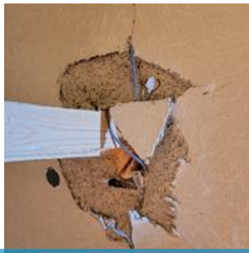
Failed Panel – 1.625-inch thick
