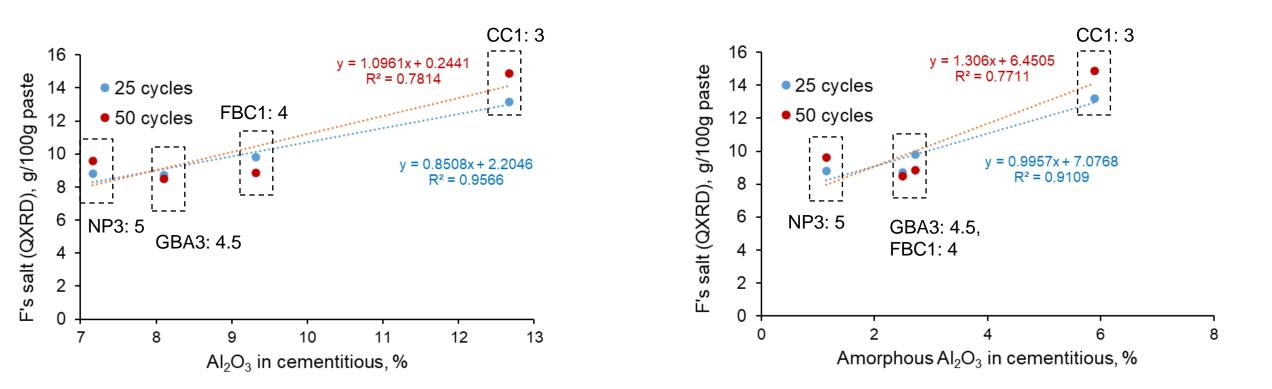
Amorphous Al<sub>2</sub>O<sub>3</sub> content in NNPs showed better correlation with ranking in the results of Scaling test (ASTM C672 scaling test temperature regime – up to 50 temperature cycles of -20°C to + 20°C, exposure to 3% wt. CaCl<sub>2</sub> solution).
