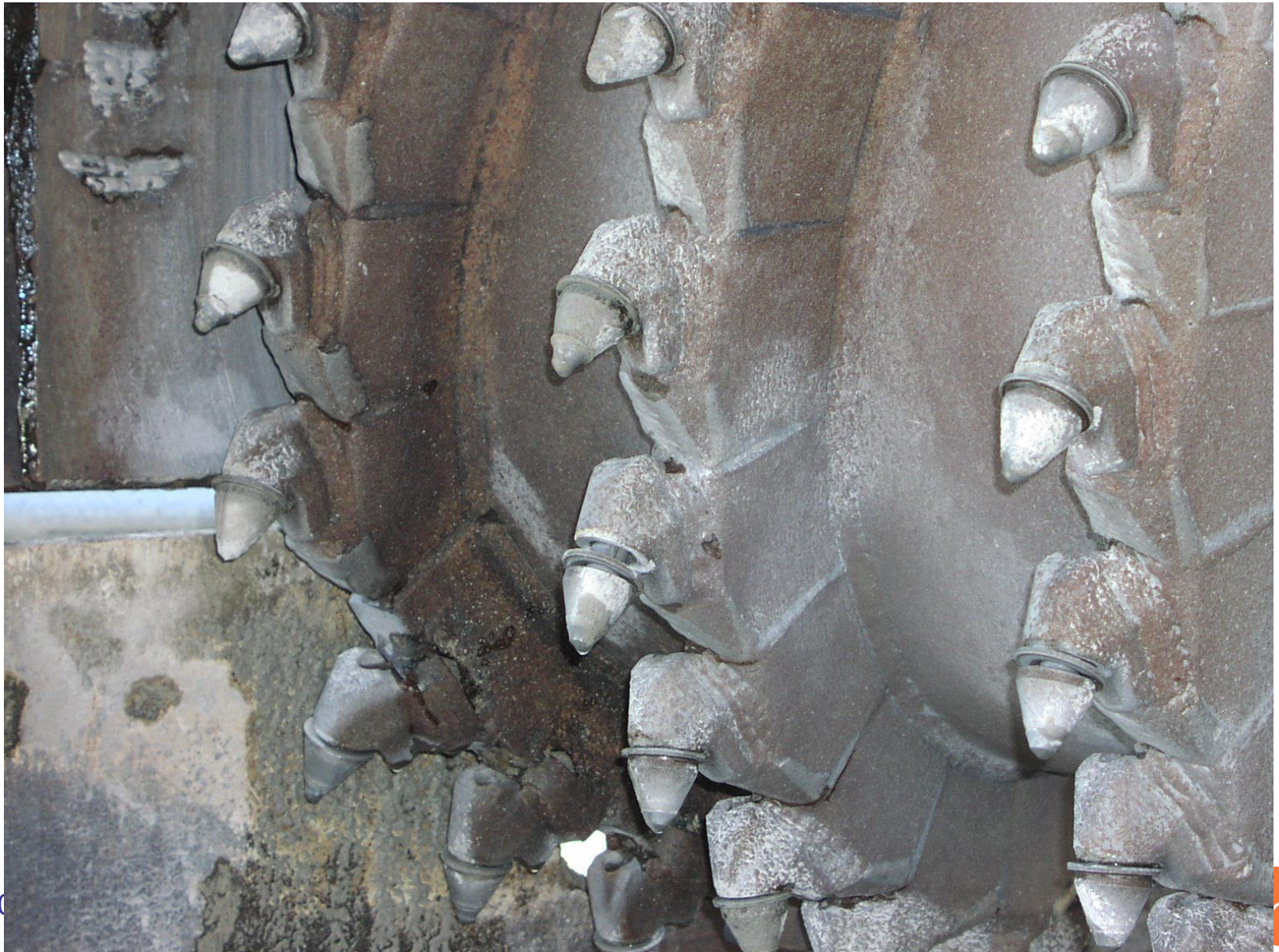
Fig 5, Micro milling heads do less damage
