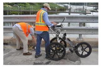
Radar testing of bridge deck. Photo: Schumacher.
