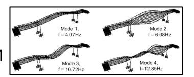
First four modes of a bridge. Source: Siringoringo et al., 2013
