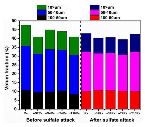
After the sulfate environment the samples shows lower porosity due to formation of expansive product
