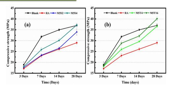
Compressive strength after 3-, 7-, 14- and 28-days of curing age of (a) NS (nERa) (b) NT (nERa) cement mortar samples.
