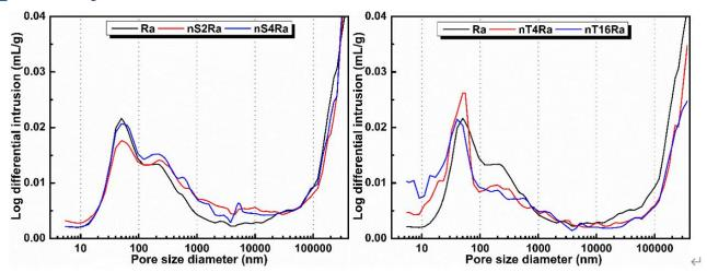
MIP results of 28 days of curing age mortar samples (after immersion in 5% Na<sub>2</sub>SO<sub>4</sub> solution)
