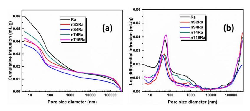
Fig.3 MIP results of cement mortar samples after 28 days of curing age
