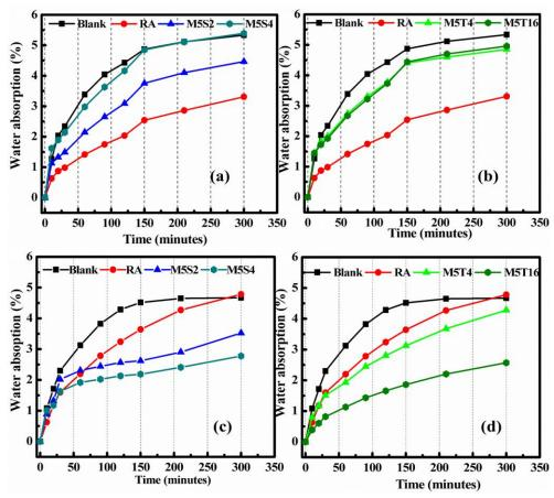
Water absorption rate % (a) NS sample after 7-days (b) NT sample after 7-days, (c) NS sample after 28-days (d) NT sample after 28-days.
