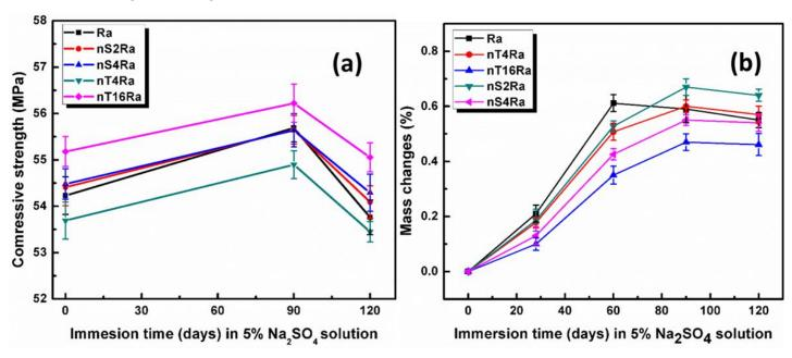
Weight and strength changes after 120 days in Na<sub>2</sub>SO<sub>4</sub> solution
