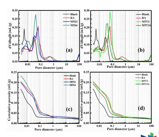
Mercury intrusion porosimetry curves for (**a**, **c**) NS and NT (**b**, **d**) cement paste samples.
