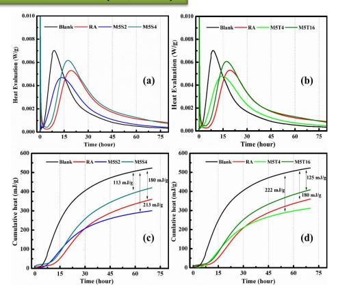
Thermal calorimetry results of (a,c) NS (nERa) samples (b,d) NT (nERa) samples.
