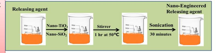
Mix proportion of nano-SiO<sub>2</sub>, nano-TiO<sub>2</sub> and RA for neRA preparation.
